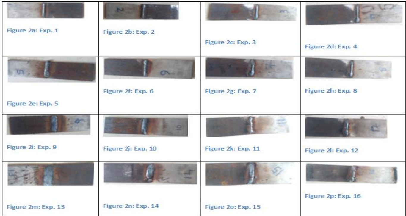
Figure 2: Based upon L 16 orthogonal array 16 welding experiments are performed
